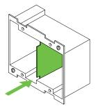
Install gang boxes that include vertical partitions (available at local electrical distributor) unless Class 2 circuit conductors are installed in accordance with 725.41 Class 1 Circuits.
